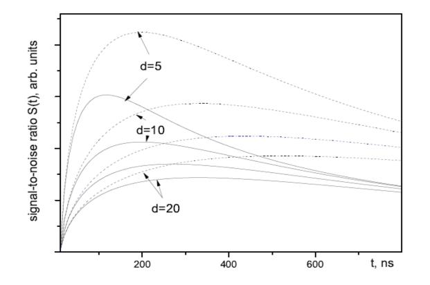
Figure 4. Dependence of the signal-to-noise ratio  $S(t) = \Delta/\sigma$  (in arbitrary units) on the measurement time gate t, for a set of inter-mirror distances d = 5(5)20 cm, mirror reflectivity R = 0.998 (solid lines) or R - 0.999 (dashed lines), and laser pulse length  $\tau_L = 20$  ns.
